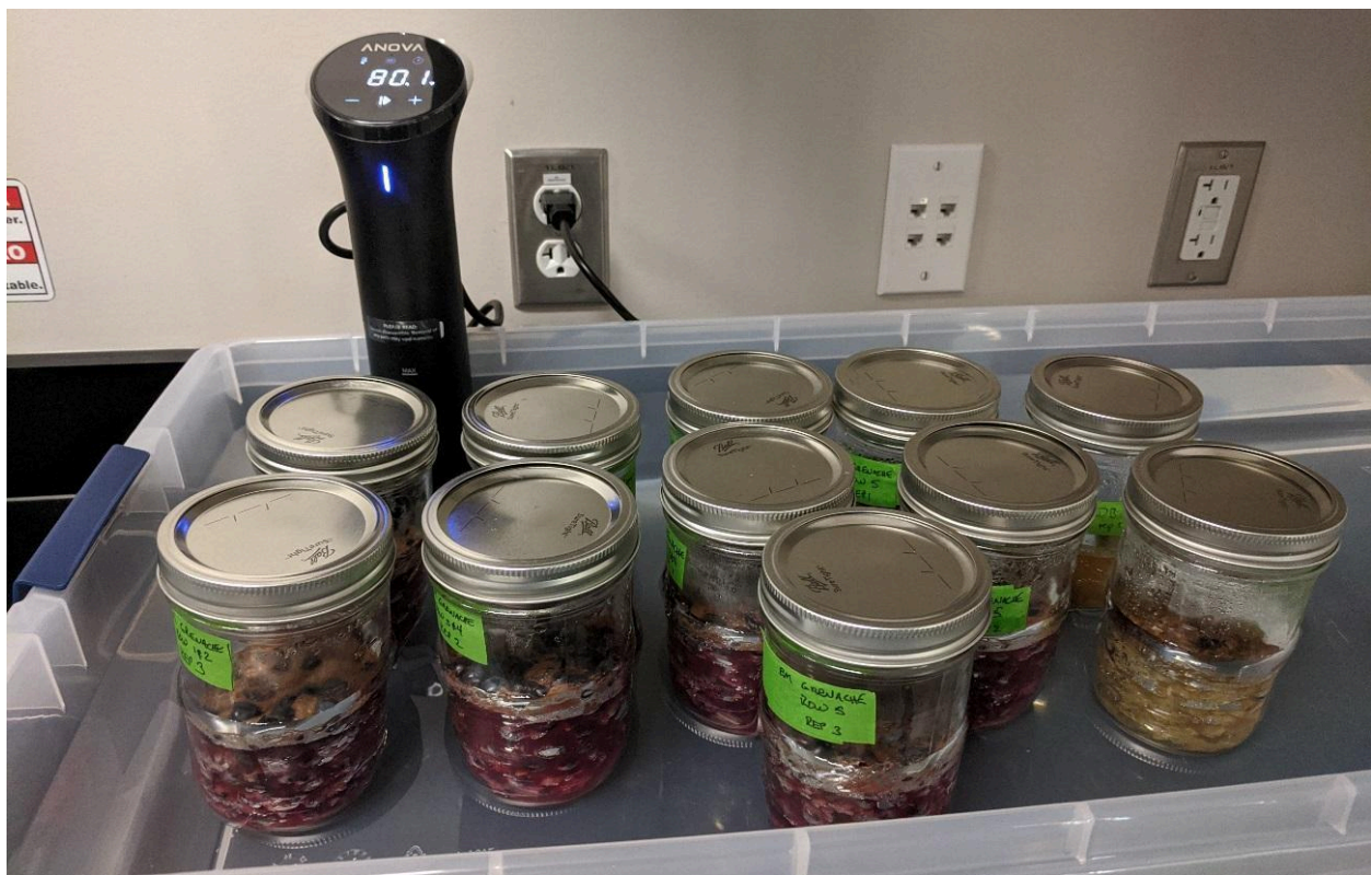
Figure 1 Under-the-bed storage box set up as a nano-scale fermentation water bath, with sous vide machine for temperature control. These are 16 oz. canning jars, with lids and bands loosely applied to allow CO 2 to escape.
